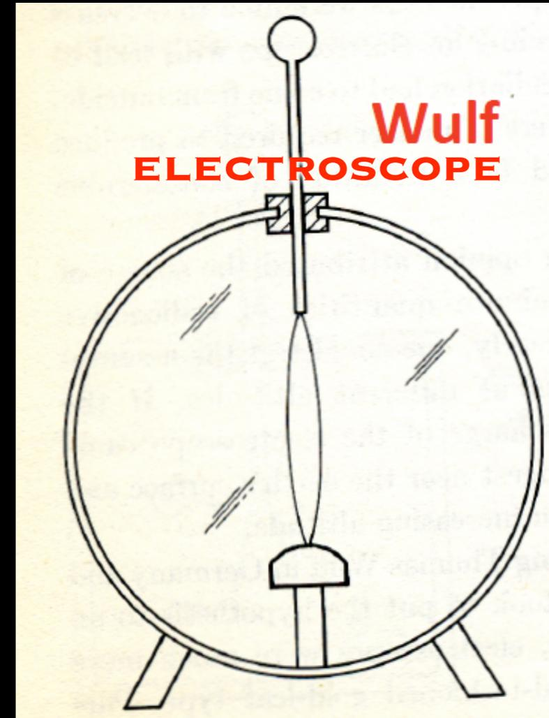
When an electroscope is given an electric charge, the leaves (or wires) repel each other and stand apart. Radiation can ionize the air in the electroscope and allow the charge to leak away: leaves or wires slowly come back together.
