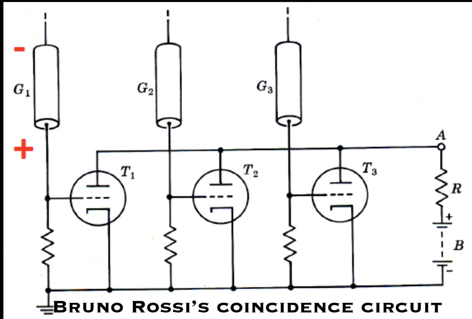
It consisted of two or more triodes with the plates connected in parallel. The grids were coupled to the G-M counters. When the grids of the triodes were simultaneously driven to a negative potential by the coincident discharges of the 3 counters, the current would stop and a pulse appear at the plates.
