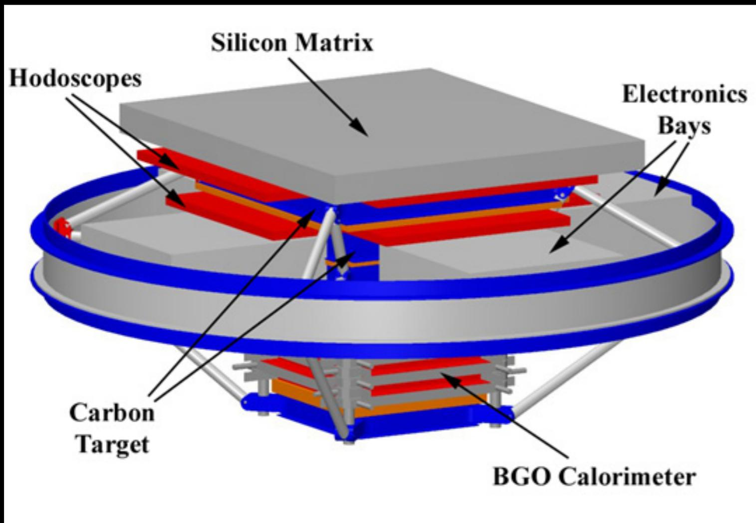
Charge measurement with silicon detectors
