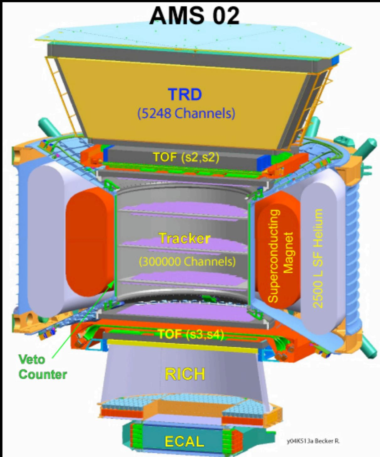
Velocity and charge measurement: Time of Flight (scintillators)
