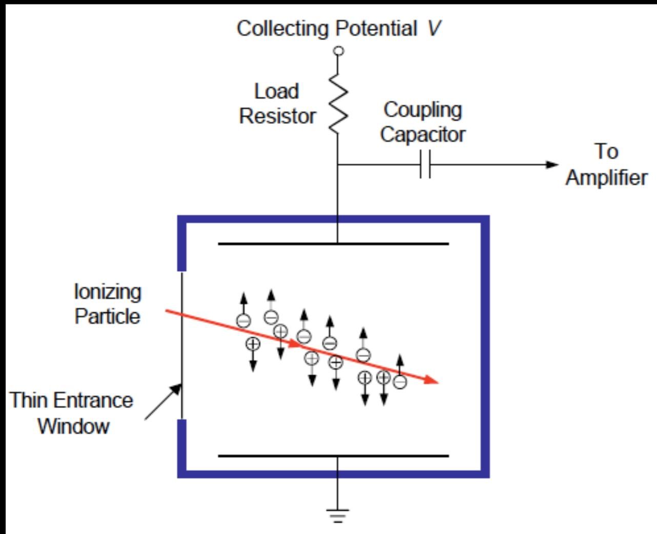
A particle passing through a gas-filled counter will ionize the gas along its path
