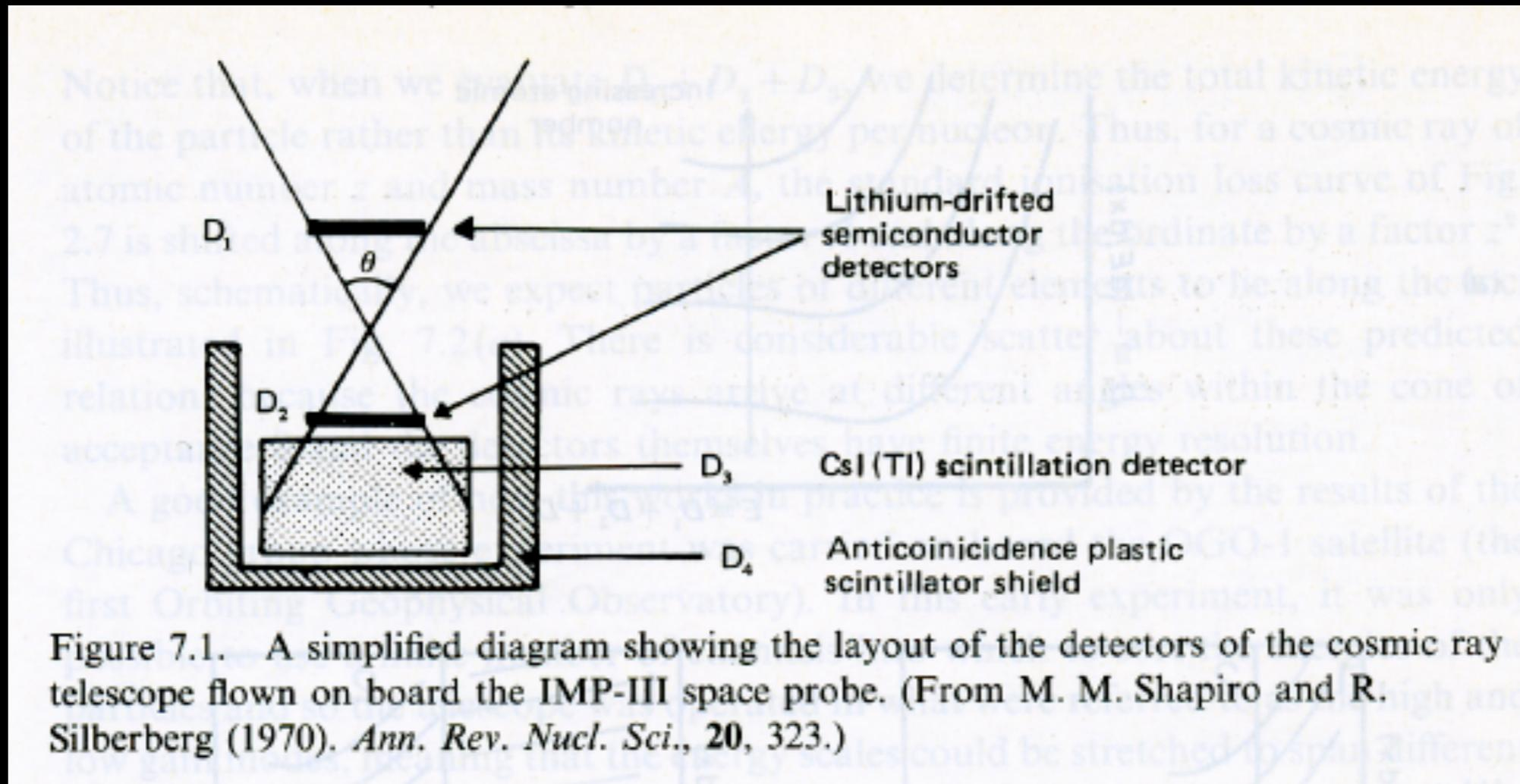
**Ionization detectors (D1, D2) on top (to register the passage of the particle, to give the “geometry” of the detector, and to measure  $dE/dX$ )**
