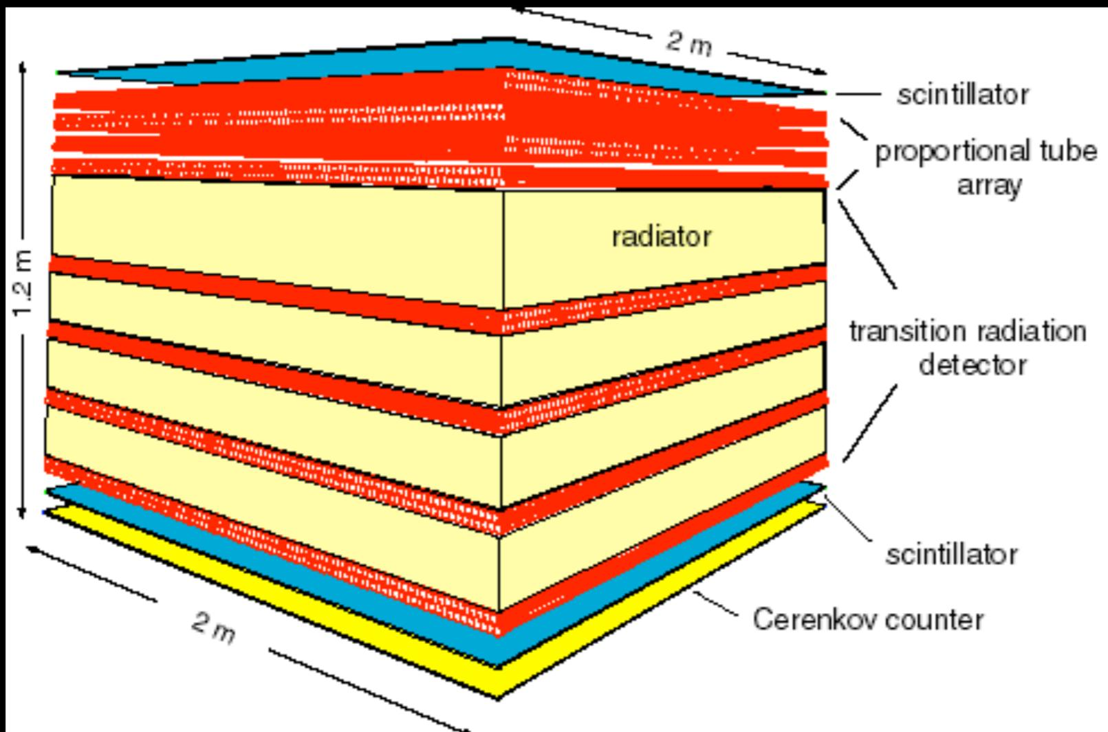
Charge measurement: 2 layers of scintillators and 1 Cherenkov counter
