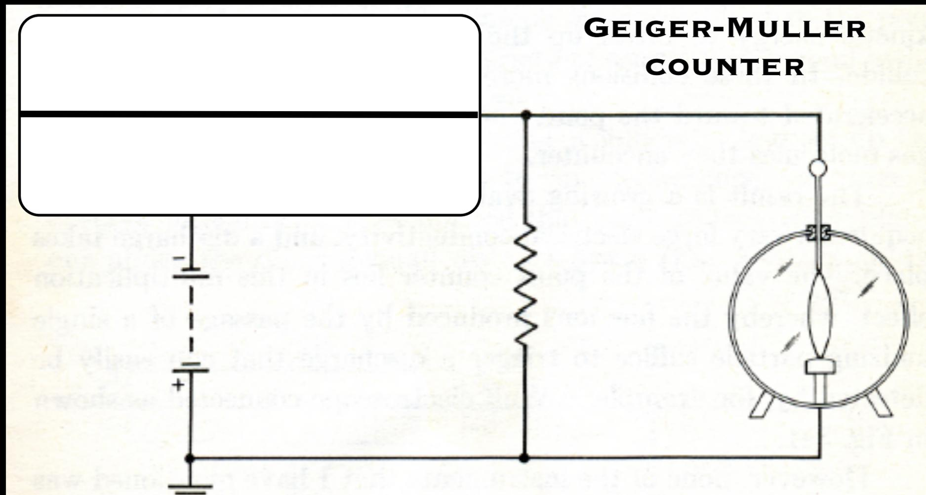
The G-M counter is easy to build, it is more stable than the point counter, and can be made in a variety of sizes. It became a crucial instrument to detect cosmic rays
