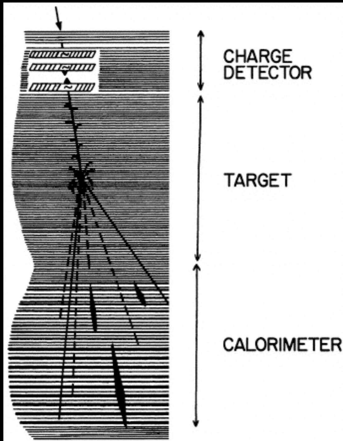
Charge measurement with thick emulsions: charge from the darkness of the track in the emulsion (ionization)
