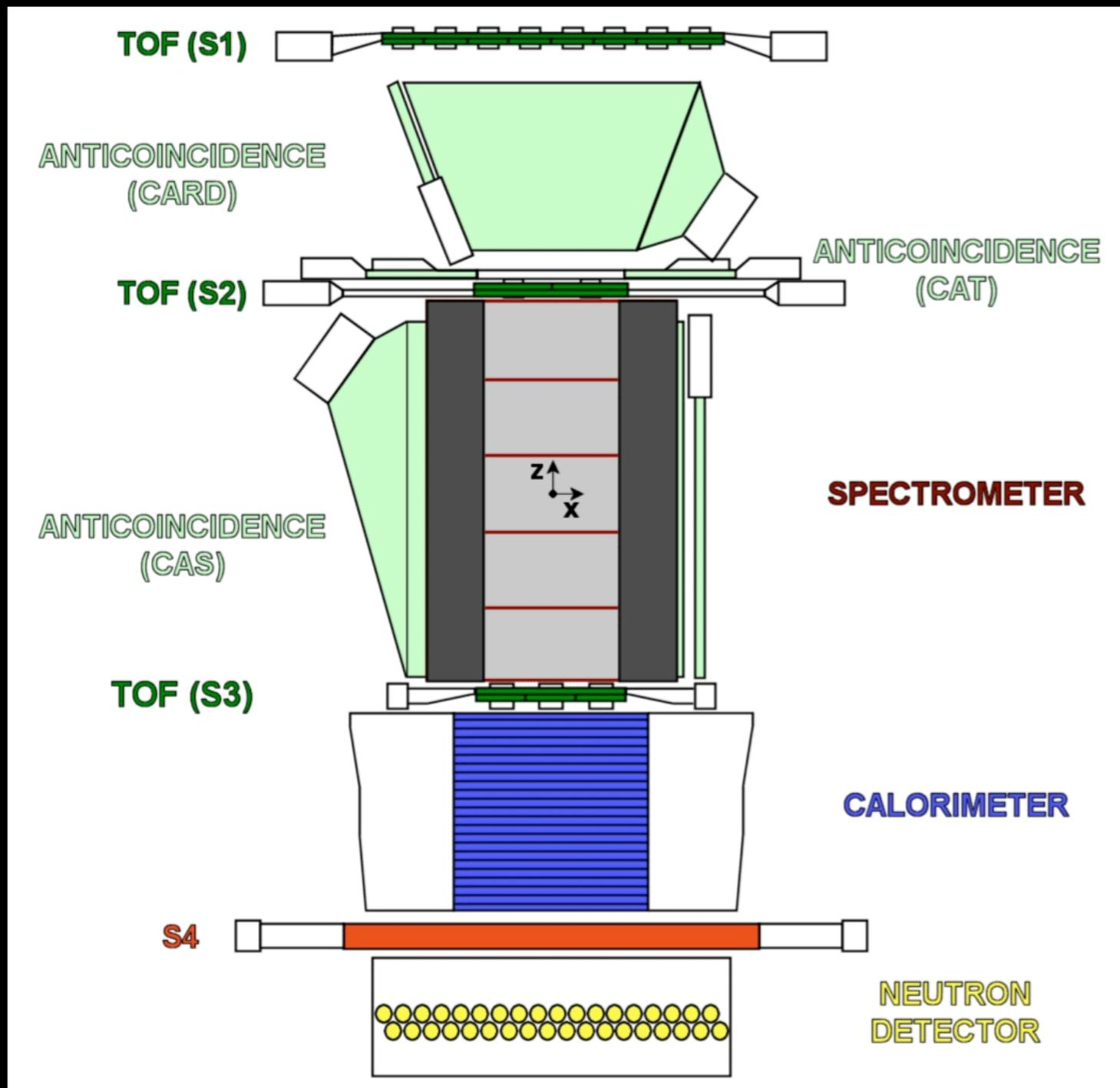
Mass and charge measurement: Time of Flight (scintillators)
