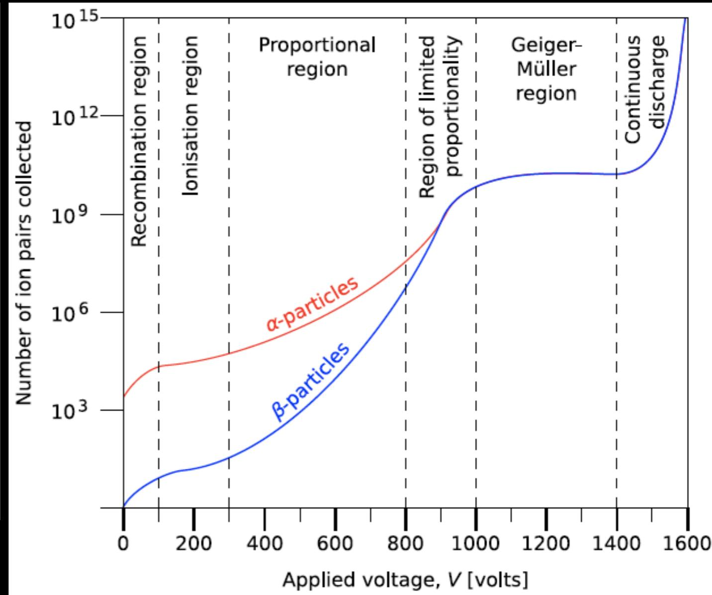
The charge  $Q$  collected (amplitude of pulse) depends on voltage  $V$ .
