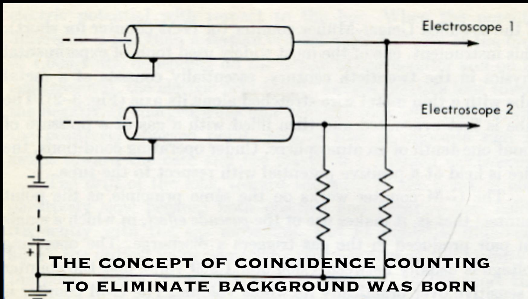
A milestone in the history of cosmic rays and their detection. For the first time, physicists had tried to determine the nature of CRs experimentally. By inserting absorbers (lead, gold) between the counters (and still finding coincidences) they concluded that “a corpuscular radiation was detected...unlikely to be a gamma-radiation...”
