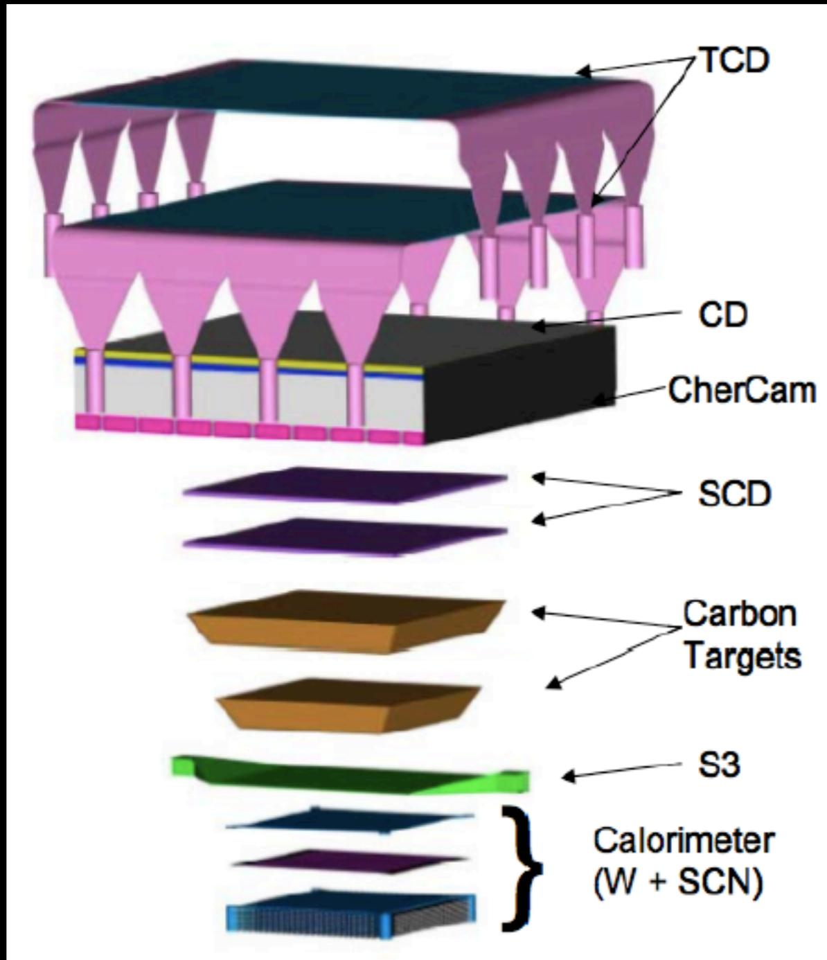
Charge and velocity measurement with Timing Charge Detector (TCD, scintillators), Supplemental measure of charge by Cherenkov Detector (CD), Cherenkov Camera (CherCam) and Silicon Charge detector (SCD)
