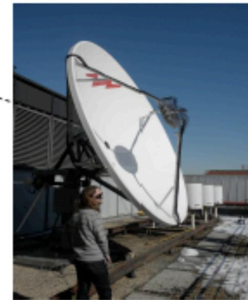
**MIDAS/AMBER:** use a parabolic dish reflector instrumented with an array of feeds, 'Radio fluorescence'.
