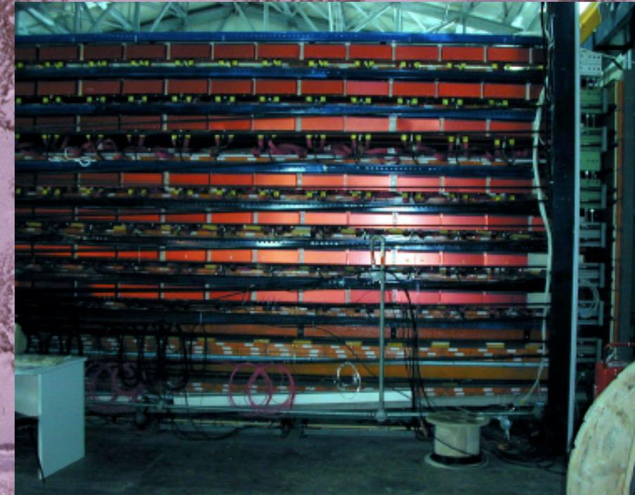
**Calorimeter at the center: muon tracking, hadron measurement**
