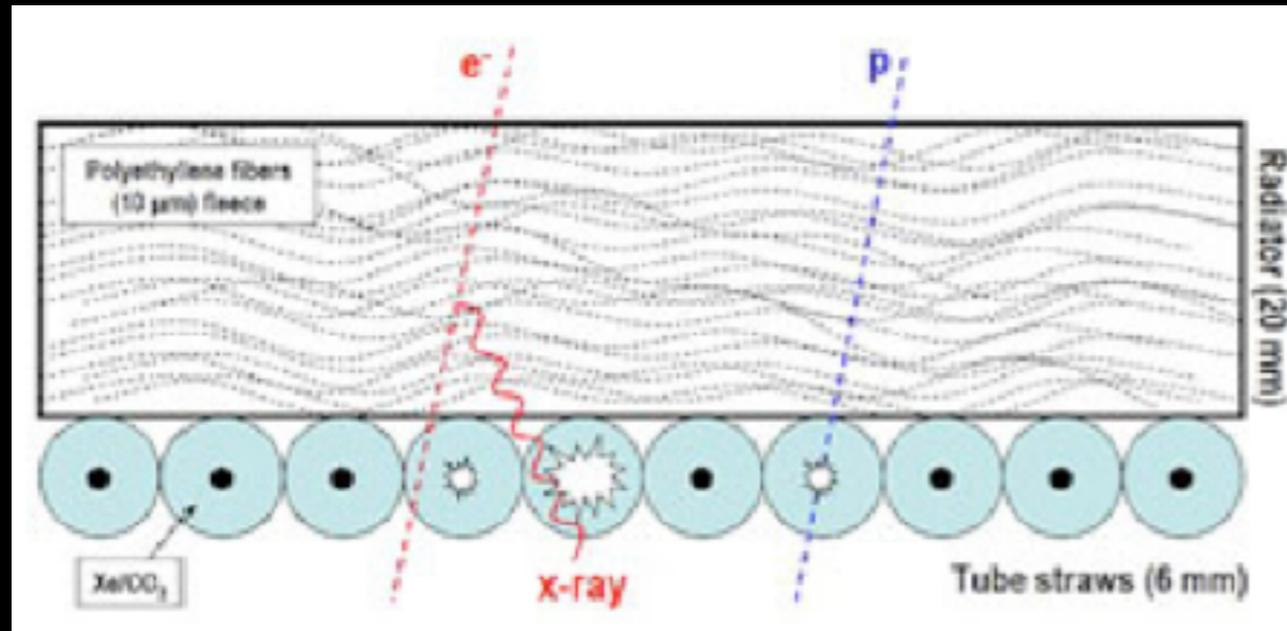
PRINCIPLE OF DETECTION OF TRANSITION RADIATION DETECTORS
