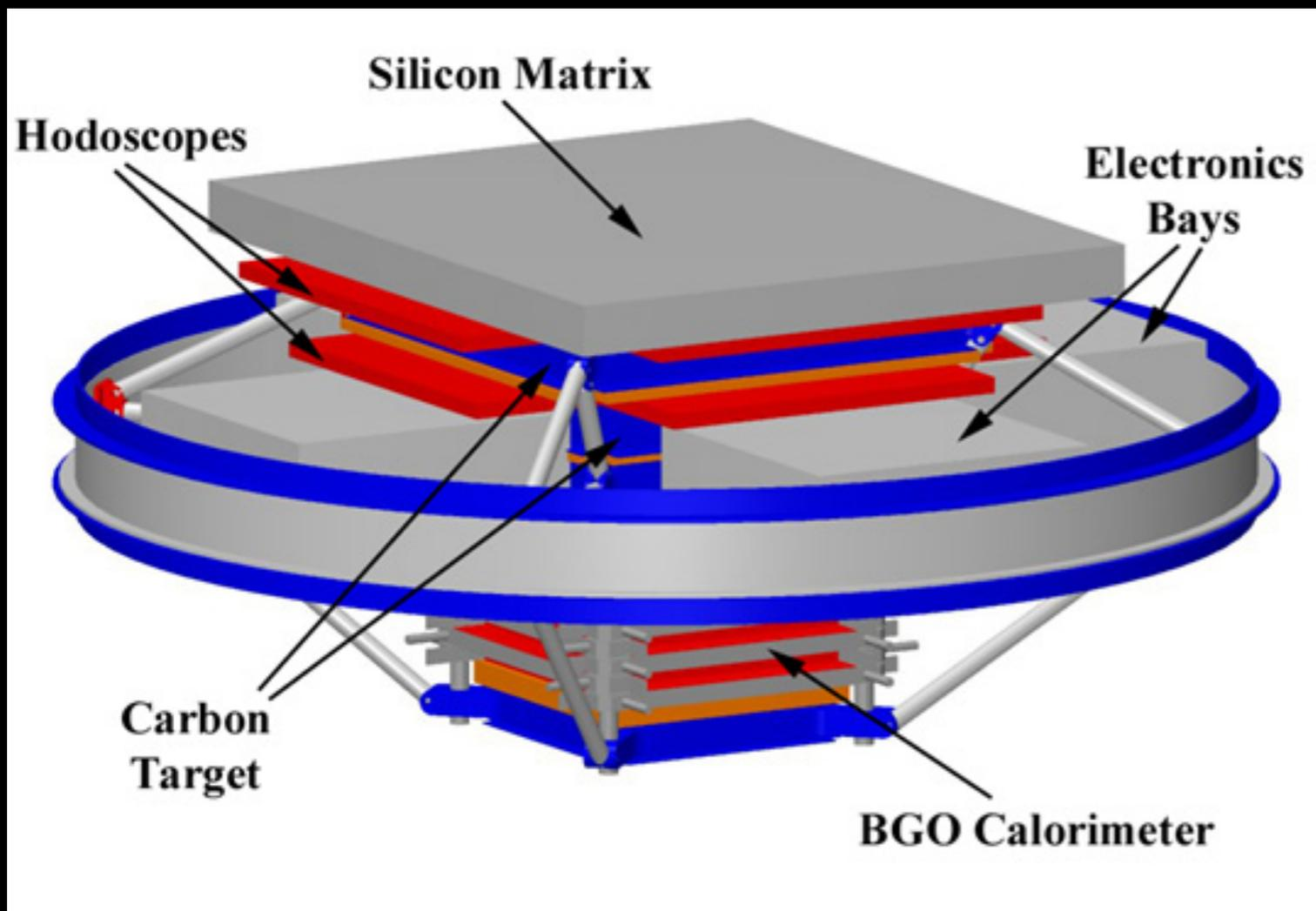
Charge measurement with silicon detectors
