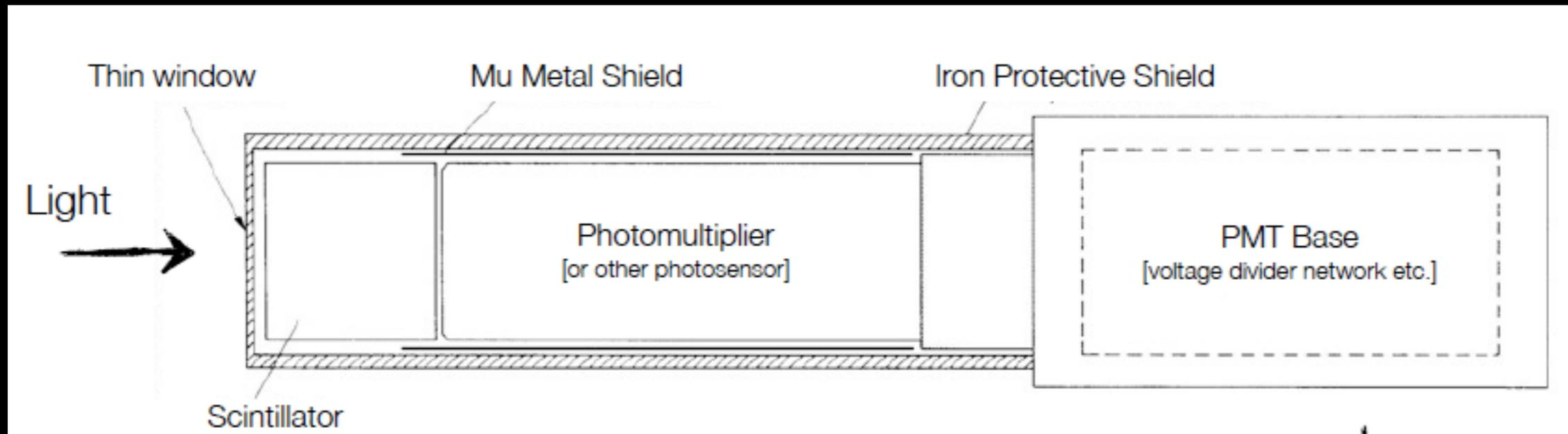
SCHEME OF A SCINTILLATION + PMT DETECTOR
